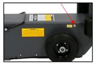
6. Repeat steps 1 to 5 checking oil level at step 5 until the rams extend smoothly to full extension and the air motor stalls.
